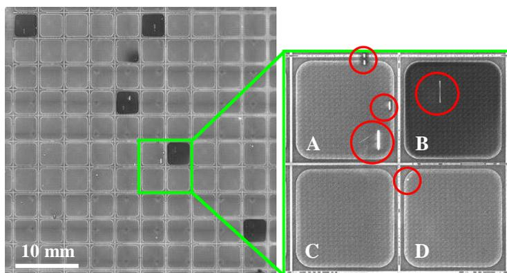
Fig. 2 PL image of a partially processed wafer with 6.5 kV pn-diodes after p-implantation and high temperature annealing. The magnified region shows four diodes of which only device C is defect-free. On the other hand, devices A, B and D show clearly visible defects in the PL imaging and therefore exhibit a significantly increased probability of bipolar degradation.
