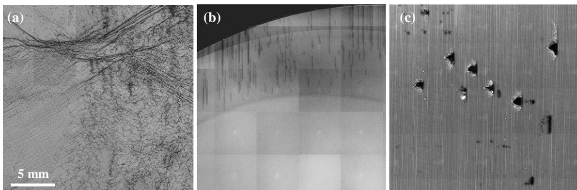
Fig. 1 Examples of typical DLS images of n-type 4H-SiC wafers: PL image of a substrate with a high TD density (a), substrate with a SF cluster at the wafer edge (b), and an epilayer with SFs, BPDs, ingrown particles and pronounced step bunching.
